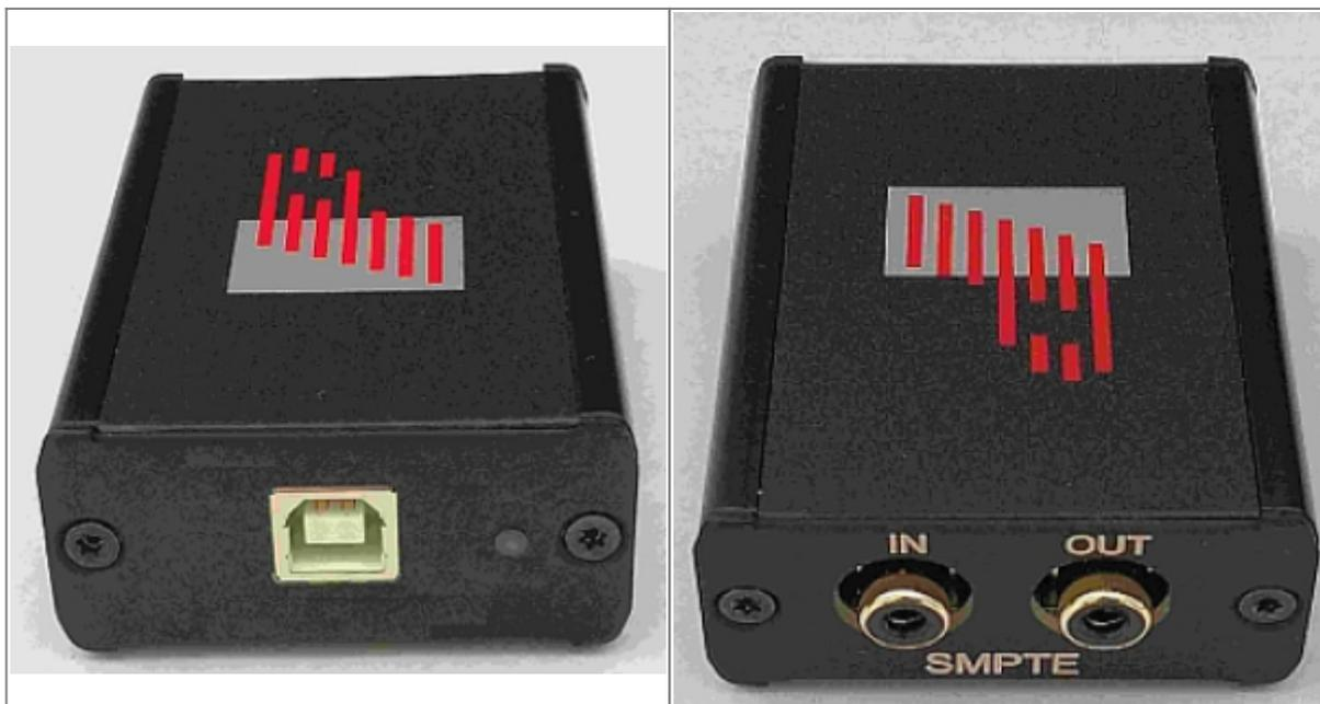
On one side we have a USB port, and an RGB status LED, On the other side we have RCA input and output for our Audio LTC, this is slightly different then the TC2000 as the TC2000 had 3 leds on the USB
