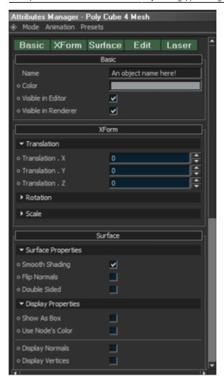
The Attributes Manager is differs in settings from each object you select. When possible the Attributes Manager is where you are able to set laser options for each individual object, and also allows you to specify an amount of segments to an object if the object isn't converted to an edible mesh yet.
