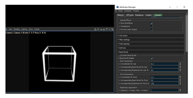
**Beam Brush Enable** must be checked for any of the other settings on this panel to have affect on the rendered object.
