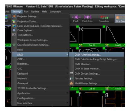
DMX (along with other 512 protocols) can be setup here, including USB DMX Devices like ENTTECH USB DMX PRO devices, Streaming Data through serial port on FB4, the DMX input and output on the QM2000.net, and over the network with Art Net and sACN.
