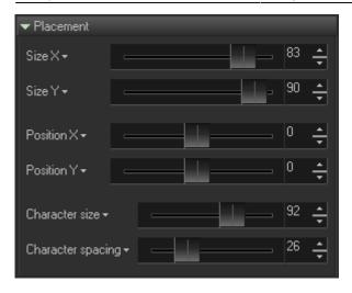
Size X and Size Y controls the overall clock size.
