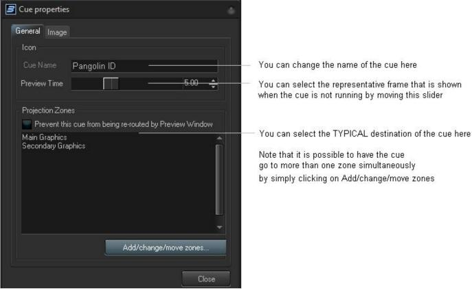
The Destination section controls the destination of the cue (i.e. where the cue will be routed once it is triggered). Note that you can specify that the cue be directed to more than one zone (i.e. laser) simultaneously, so if you check both the "Zone 1" and "Zone 2" boxes above, the cue will be directed to both lasers simultaneously.
