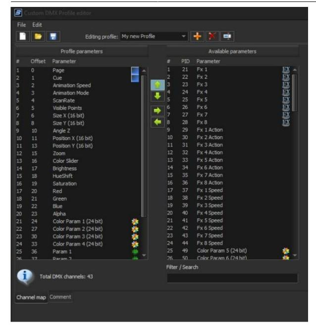
There are a number of parameters you can add. The first main block is going to be the parameters that are included inside the default DMX Server profiles. From there you have access to the Quick FX grid with FX number, Action and speed. "Color Channels", and "BEYOND Channels" These can then be added to your profile to allow for BEYOND control, or FX Control in either all areas of BEYOND, or effects baked into your profile.
