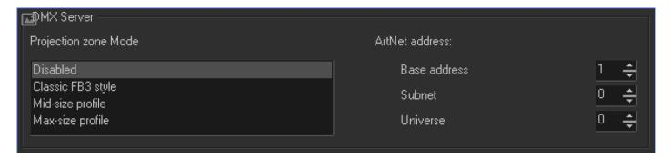
As soon as the Mode is selected, the Projection Zone is ready for external control. Under the hood, the Projection Zone has it's own Cue Player that performs the playback. All the output from the player goes to the corresponding Projection Zone. Keep in mind, a Cue may contain different types of content, from simple animations to multi-projector shows. Do not use multi-projector show Cues, as these will overload the Server's output.
