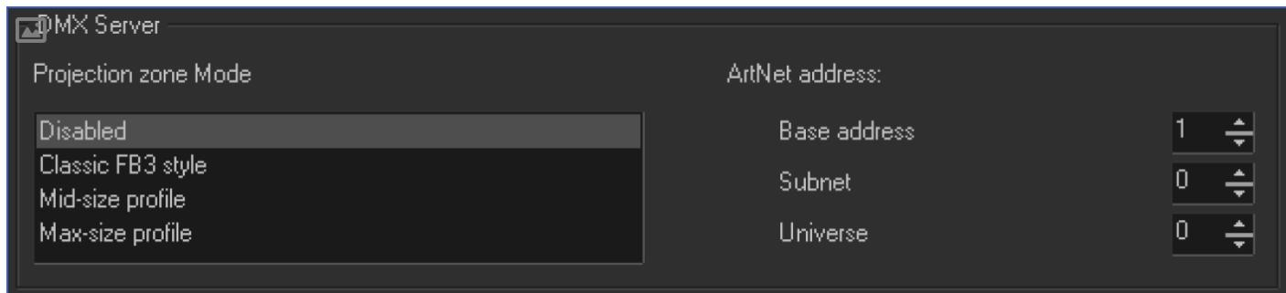
As soon as the Mode is selected, the Projection Zone is ready for external control. Under the hood, the Projection Zone has its own Cue Player that performs the playback. All the output from the player goes to the corresponding Projection Zone. Keep in mind, a Cue may contain different types of content, from simple animations to multi-projector shows. Do not use multi-projector show Cues, as these will overload the Server's output.
