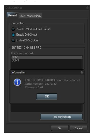
First specify whether you want to use DMX Input or Output using the "Connection" portion of the dialog box. After that, specify the COM port where the DMX-to-USB controller is connected.
