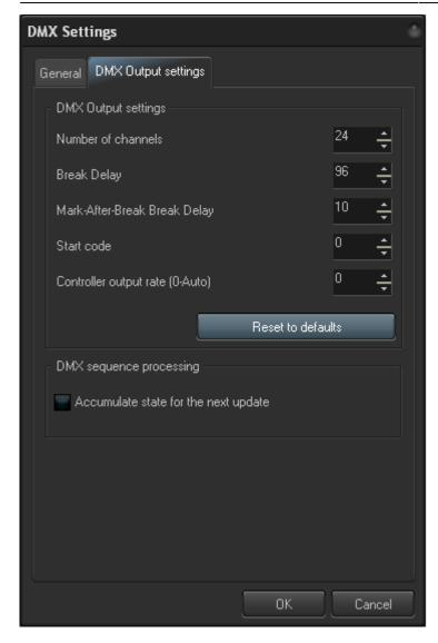
The DMX Output settings also has advanced controls that allow you to control the timing of the DMX signal. Generally the default values should work well, and you would only need to make adjustments to these settings if you suspect data corruption or incorrect DMX signal receipt.
