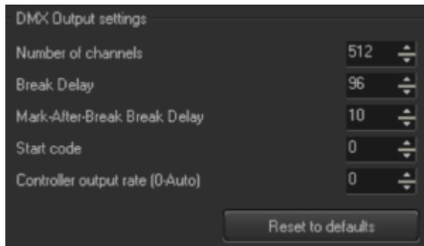
Additional DMX Output settings are also located here and have advanced controls that allow you to control the timing of the DMX signal. Generally, the default values should work well, and you would only need to make adjustments to these settings if you suspect data corruption or incorrect DMX signal receipt. You also have the ability to reset any of your changes back to their default values.
