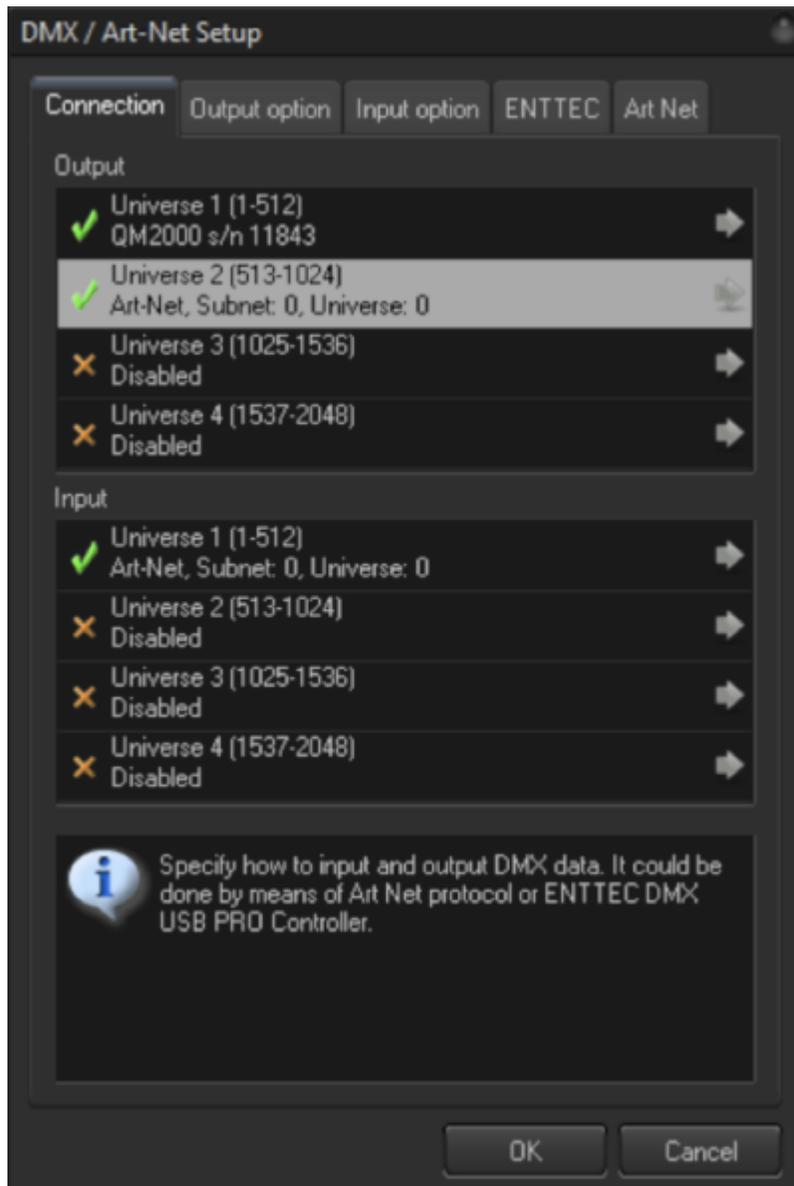
DMX IN comes into BEYOND by means of ArtNet protocol, the Enttec DMX PRO USB controller or Pangolin QM2000 hardware. To setup the communication, go menu Settings→DMX/ArtNet Settings.
