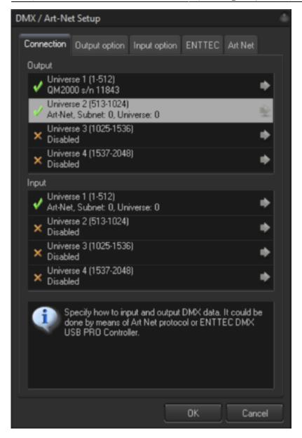
DMX IN comes into BEYOND by means of ArtNet protocol, the Enttec DMX PRO USB controller or Pangolin QM2000 hardware. To setup the communication, go menu Settings DMX/ArtNet Settings.
