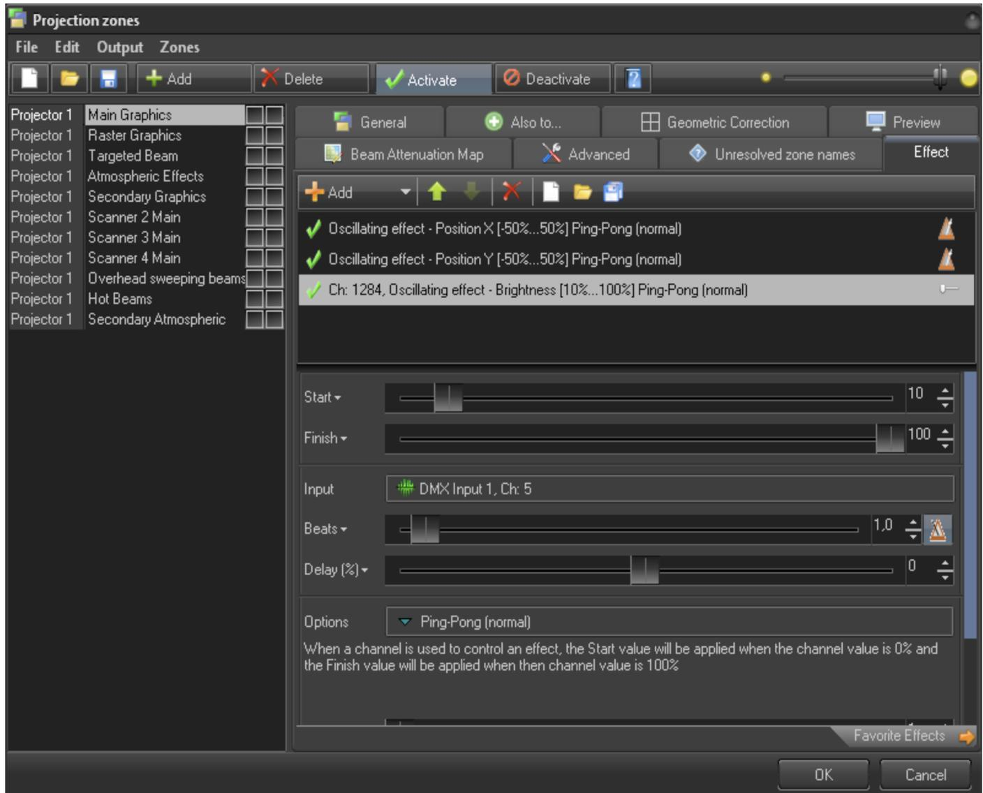
Using DMX is possible with any Effect, but let's consider Projection Zones, as that serves as a good example in the context of external control of BEYOND. The Effect tab shows the standard effect editor. Click on the "Input" button. In the "Input setup" dialog select DMX Input and the number of channels. After this, the effect item will follow the DMX channel value. The value of the channel is mapped to the range (from Start to Finish) specified in the effect.
