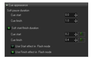
**Soft pause duration** - **cue start** - defines the time (in seconds) for the amount of time it takes to accelerate the cue to full playback speed. Instead of an immediate pause and cue playback start, BEYOND can start the cue "softly", or slow down/speed up the playback of the cue during the specified time.
