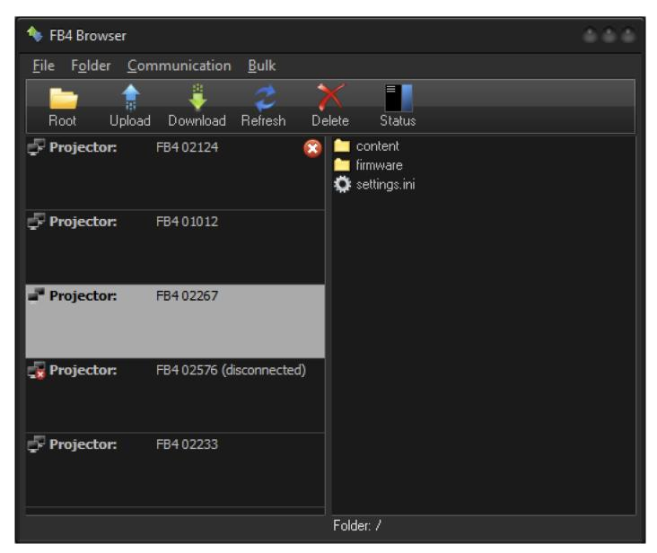
The FB4 needs to be connected to BEYOND/QS software to enable operations with the SD card. The left side of the window shows a list of connected FB4 hardware. The list indicates the Projector serial or name, connection state, presence of errors and the upload/download progress (if there are active operations).
