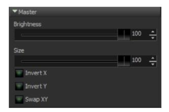
Allows adjusting of the Master Brightness and Size, and Axis Invert. Master Size and Brightness influence all modes including streaming from BEYOND/QS.
