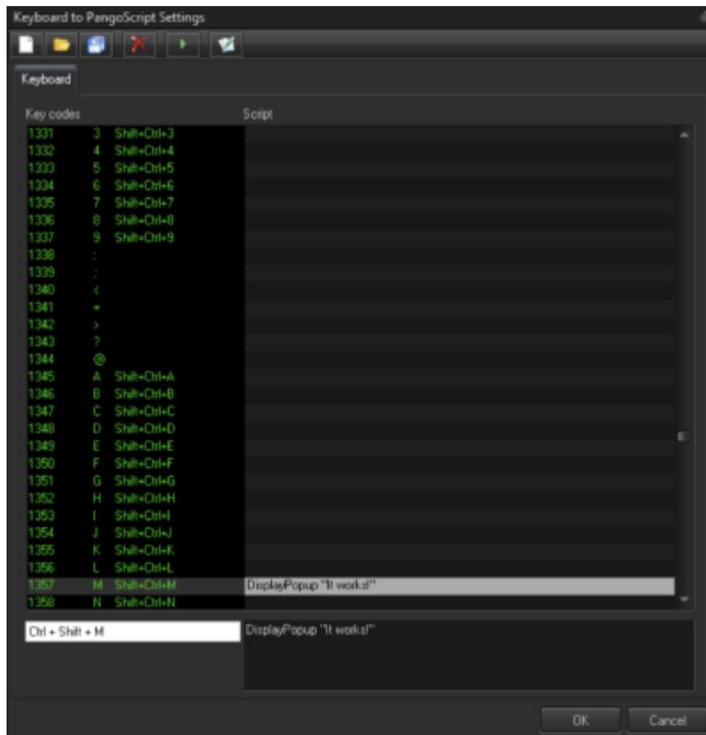
The left side of this interface will display key codes, and the right side shows the corresponding PangoScript. For quick navigation in the list, enter the key into the edit-box located at the bottom of the list. Double click on list to open the PangoScript editor. BEYOND will save the settings into a file automatically in the System folder. There is no need to save the file, just click OK.
