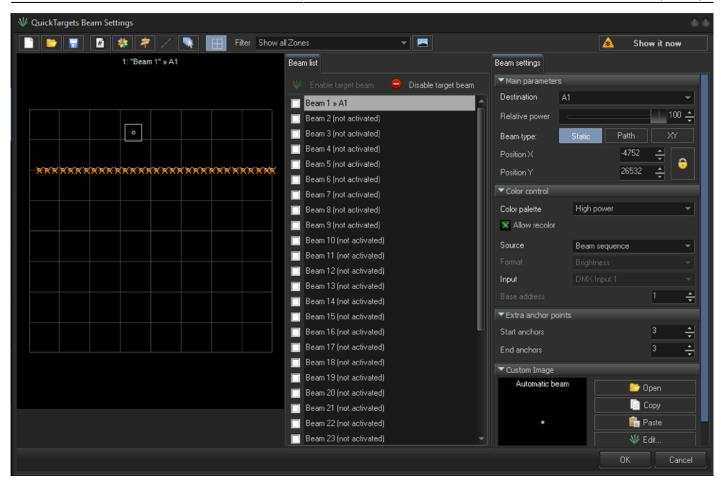
Here we have control of our beams, where we can set our destination (zone), its power, and if it Is enabled. These features work the same as they do normally In Quick Targets Beam Settings.
