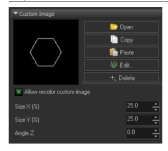
Quick Target system allow to use frame, and other images instead of just a beam. If you use custom image, then BEYOND will stop dynamic power distribution and each beam will take as much points as supposed to be in the Image.
