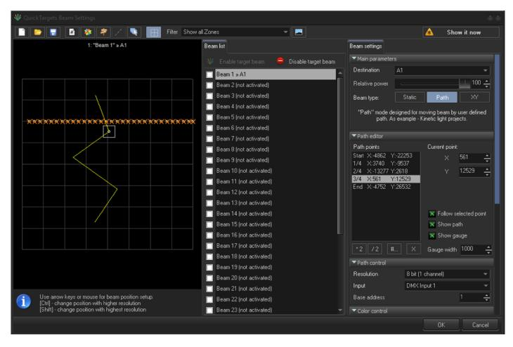
On your console, its best to put a specific kinetic fixture at its "0%" position and place your starting beam by moving it with your mouse, ensure "**show it now**" enabled. Position your beam onto the center of the ball, or whatever you are hitting. Then move your fixture to the "100%" position and do your end point.
