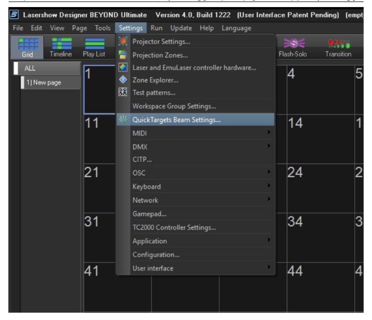
This opens the window "Quick Targets Beam Settings", where the kinetic plugin features are located.
