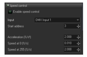
This is where we can adjust our beam movements, so the beam reacts more like a physical fixture instead of a digital position. Imagine you had a position in your programmer for your kinetics, if you clear your programmer, the balls take time to retract to their "start" position. While the DMX value instantly goes to zero. Since BEYOND is listening to DMX values directly the laser beams would return immediately to the "start" position set in the path.
