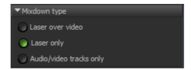
The first Setting is Mixdown Type. It defines which kind of video file you need to create – just a laser show, just a video file, or a laser over video, video. When the selected option is "Audio/Video tracks only", the File format combo box will offer several audio formats in addition to video formats. If you choose an audio file, then video portion will be ignored (if present).
