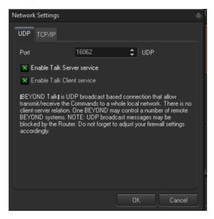
The default ports used are 16062 for UDP and 16063 for TCP. Now you need to enable the Talk server service and talk server client service in the network settings window. Open up
