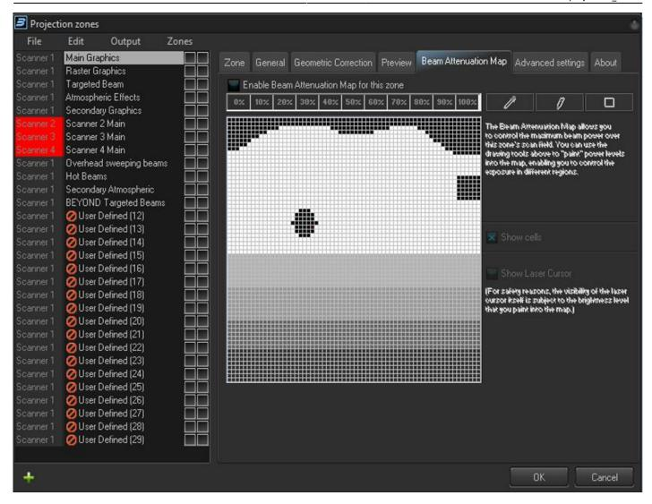
The Beam Attenuation Map is a 64 by 64 "pixel" brightness control map. Each pixel can be set to any brightness level from 0 to 100%. Rudimentary tools are provided to sample a brightness level in the map, fill the entire map with the selected brightness level, fill a rectangular area with the selected brightness level and freehand-draw brightness levels into the map.
