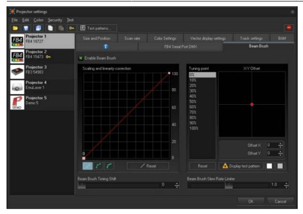
We have added a tab on the projector settings window for projectors which feature Beam Brush®. As there Is control parameters that need to be considered with a Beam Brush® projector. This tab Is exclusive to each connected piece of output hardware and is saved to the pc and can be saved to a file for future loading.
