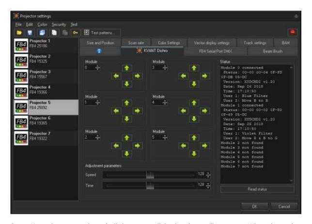
Some Kvant lasers may have built in remote dichroic mirror adjustments. When the projector has this functionality the "KVANT Dichro" tab will appear. The first step will be to click "Read Status" on the bottom left, this will read the data from the projector on which "module" is doing what inside the projector. In the above example you can see Module 0 moves Blue to Red. You can use the buttons for left right up and down to shift the mirrors to do a color convergence in the projector.
