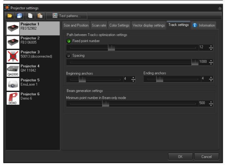
BEYOND generates special transitional (short) frames between the tracks/frames as well as between display updates. For example, if you display two cues, then BEYOND will inject a transitional path between them. The path is a blank line with a few anchor points in beginning and ending of the line.
