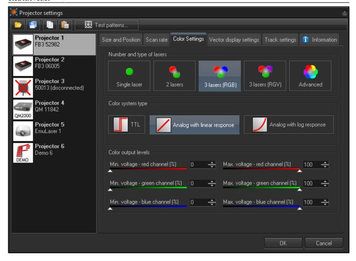
When configuring BEYOND, be sure to indicate the number of and type of lasers in your projector, along with the color modulation scheme (color system type) used with your projector. BEYOND offers a few standard modes for quick setup and an Advanced mode that provides more flexible options.
