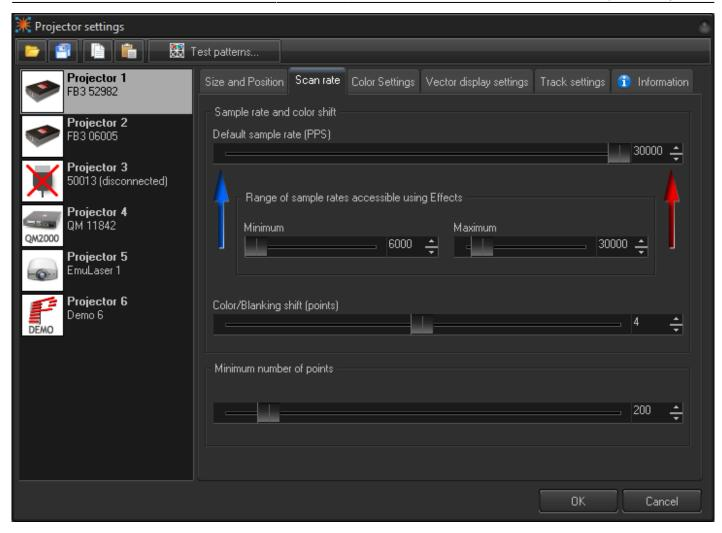
**Default sample rate** values should be tuned using Test patterns. There is direct relation between default sample rate, color shift, Sample rate, Size, and Position. Bigger size means a larger angle and as a result more time is required for motion; your Sample rate should be lower. Conversely, for smaller angles, the sample rate can be higher.
