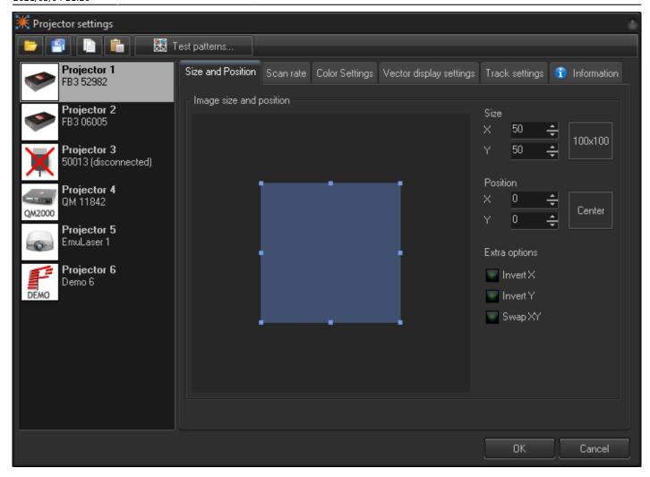
ize and Position are "global" settings of the Projector. "Global" means all Projection zones that go to this Projector will be influenced by this setting. The Projection Zone menu has Geometric correction settings which can appear to create some redundancy.
