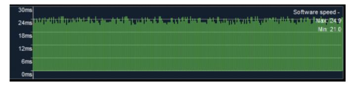
Lines ending at range of 20 .. 25ms are OK. If you see diagram like saw tooth, then this indicator of CPU overload. CPU cannot come to calculation in time. So, you see sawtooth here instead of line – this is direct indicator of CPU.
