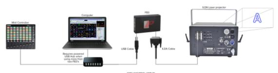
Here you can see a basic setup including an APCMINI midi console using a single laser enjector. The same principles for shared and independent control mentioned above, apply here
