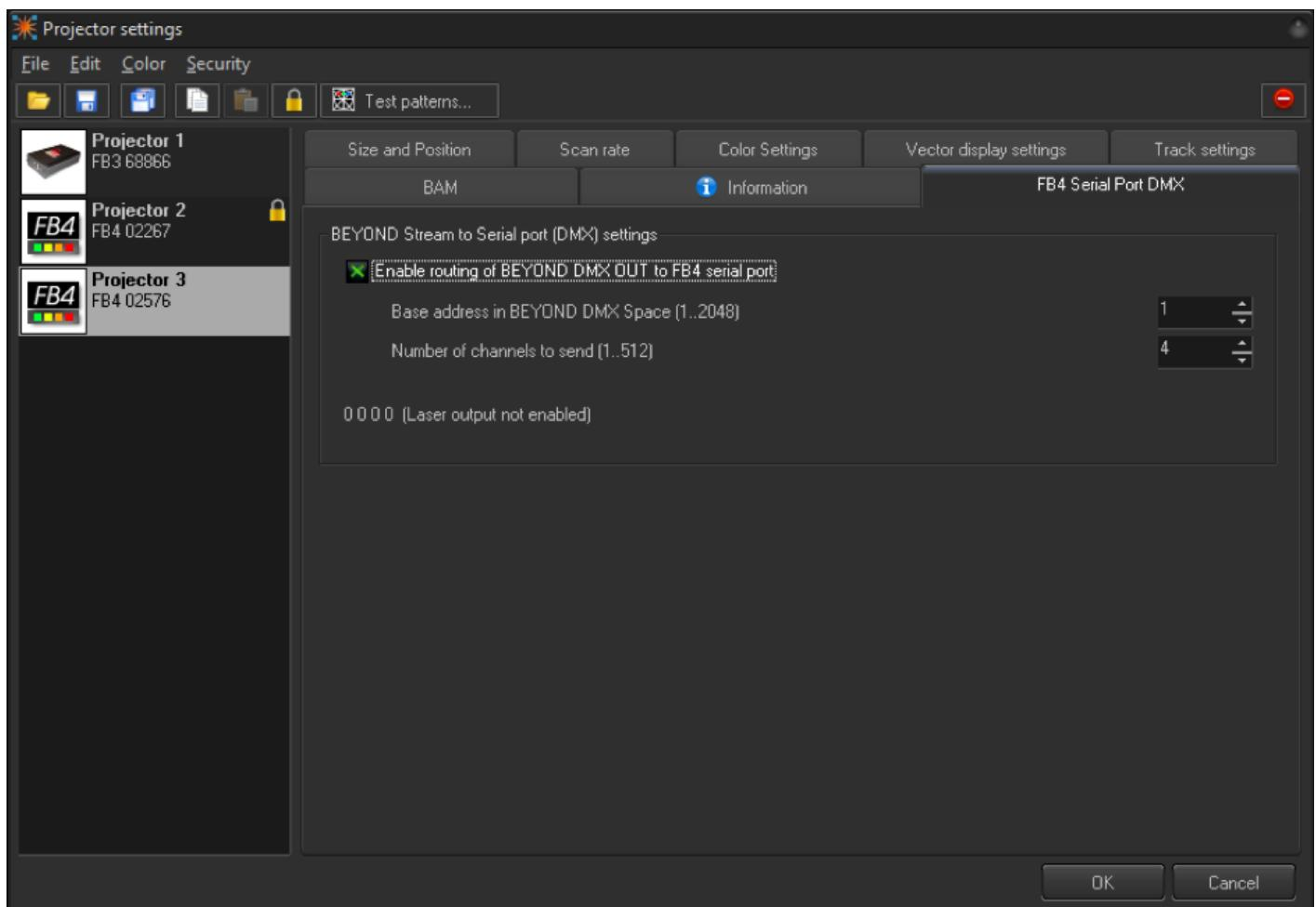
The “Base address” defines the positions of the 1st channel in BEYOND’s output DMX array. “Number of channels” defines how many DMX channel values are passed through to the serial port, so in the example above we choose base address 1 with 4 channels to send, so BEYOND will send to the channels 1, 2, 3 and 4 through the FB4.
