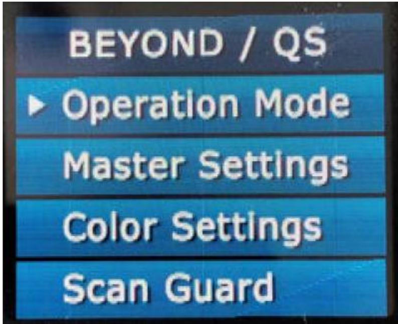
The feature is called "Scan Guard", it's designed to provide an additional method of safety so that static laser beams will be blanked as soon as laser output meets certain specific defined settings.
