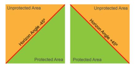
The Horizon Angle allows a Horizon Level to be rotated by up to 45 degrees in either direction, which could be useful if the laser projector is not level, being mounted on an angled truss for example.
