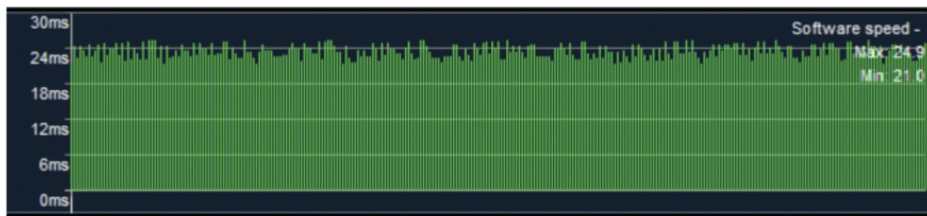
Lines ending at range of 20 .. 25ms are OK. If you see diagram like saw tooth, then this indicator of CPU overload. CPU cannot come to calculation in time. So, you see sawtooth here instead of line - this is direct indicator of CPU.
