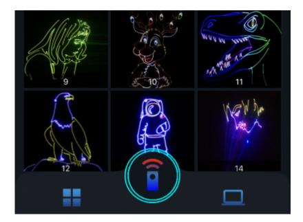
At the very bottom of the window, you will see a button in the middle. Tapping on his button will bring up the Live Controls section of the app. This allows you to adjust the Size, Position, Rotation, Color and Playback speed, in a way very similar to how it works in QuickShow and BEYOND(PS: Hue Shift and Saturation in Color is only available in BEYOND).
