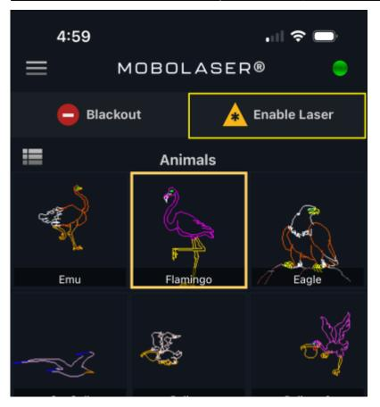
On the top/right of the application window, there is an Enable Laser button. Pressing this will toggle the state of whether the laser will project content or not.
