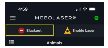
On the top/left of the application window, there is a Blackout button. Pressing this button at any time will immediately cease all laser output.
