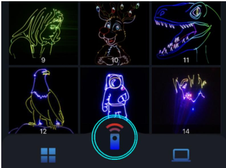
At the very bottom of the window, you will see a button in the middle. Tapping on this button will bring up the Live Controls section of the app. This allows you to adjust the Size, Position, Rotation, Color and Playback speed, in a way very similar to how it works in QuickShow and BEYOND (PS: Hue Shift and Saturation in Color is only available in BEYOND).
