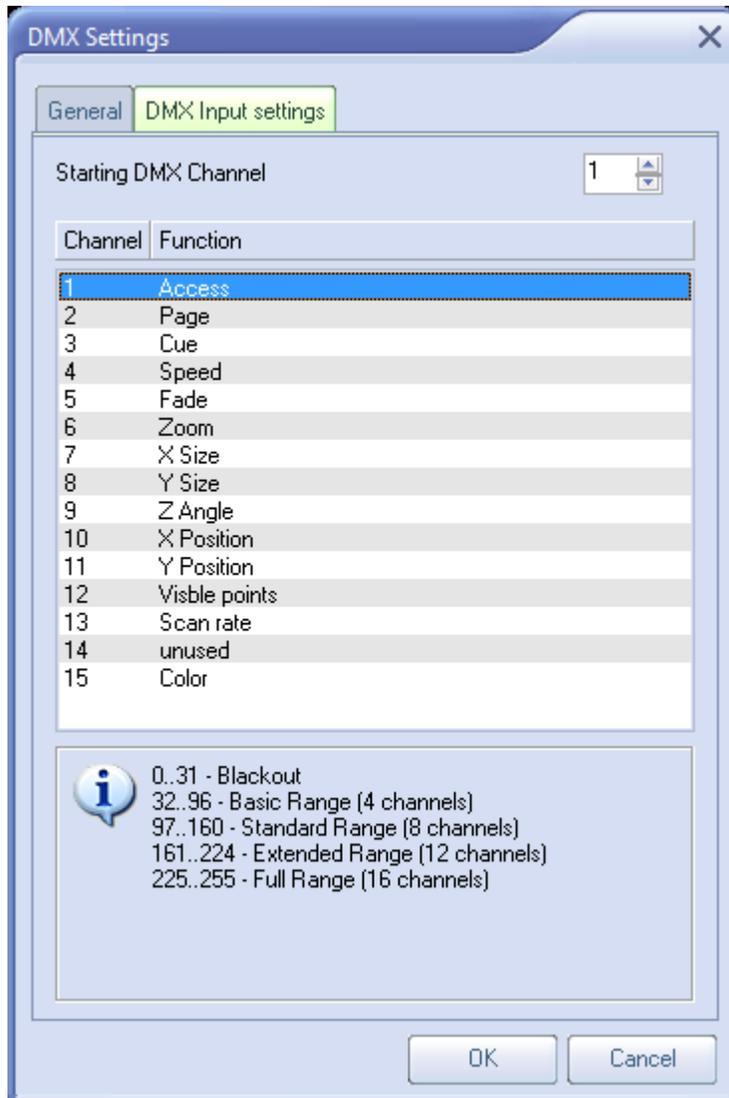
As shown above, the DMX Channel Assignment for QuickShow is exactly the same as that of the FB3-SE DMX daughter board. This allows external controllers that are already familiar with the FB3 to easily control QuickShow in the same way and providing the same results.
