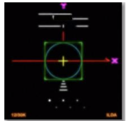
Color shift too high: Horizontal lines shifted too far right
