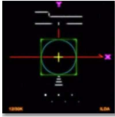
Color shift correct: Horizontal lines approximately centered
