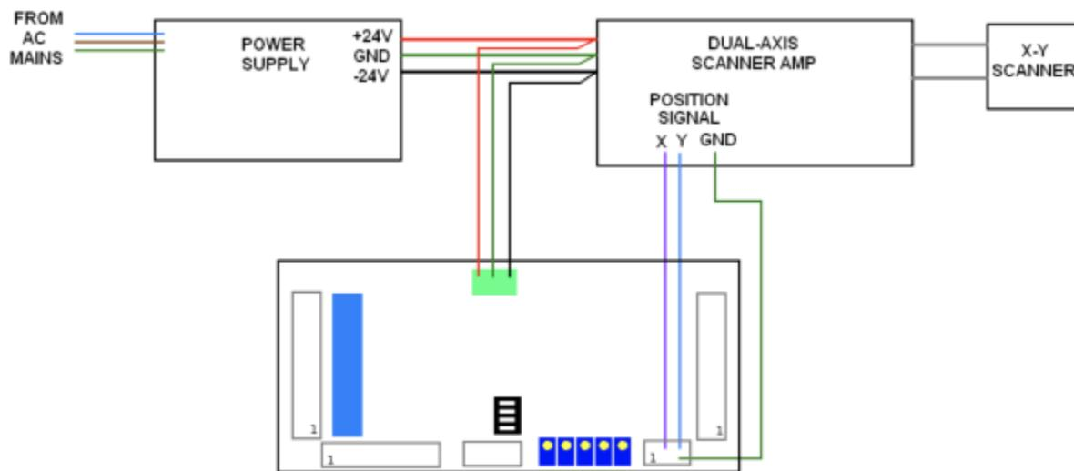
If you are using a one dual-axis scanner amplifier, the recommended connections are shown below:
