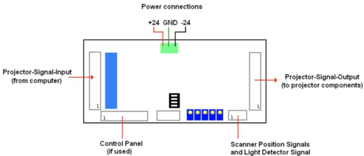
The general layout of PASS is shown above, with connectors identified.
