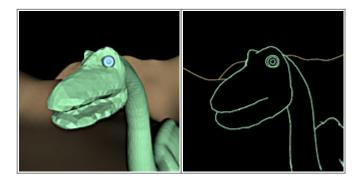
Obviously if the laser tries to scan all of these short runt lines, flicker might result. For this reason, Lasershow Converter 4D includes several filters to aid in the creation of smooth paths for the laser to follow.
