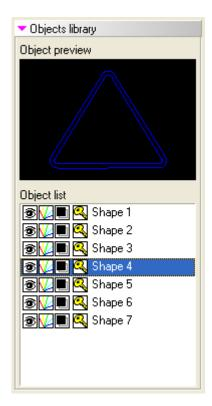
The Object Library has two purposes. First, it allows you to select and preview each object in the FLASH file. Second, it allows you to control various aspects of the rendering and laser output.
