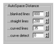
Note that in both cases, the **Straight lines** point density needs to be decreased from the default value of 300. This ensures there will be enough points placed for small details and to avoid rounding in the images.
