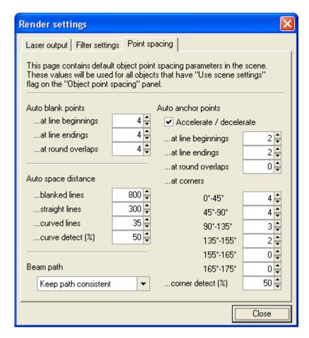
**Note**: The numbers shown above are the default values. They are optimized for scanners tuned to the ILDA 30K standard, when running at a point output speed of 30,000 points per second. If you do not change any of the numbers, objects will use the default values. For more information, see the topic Scan speeds and LC FLASH.
