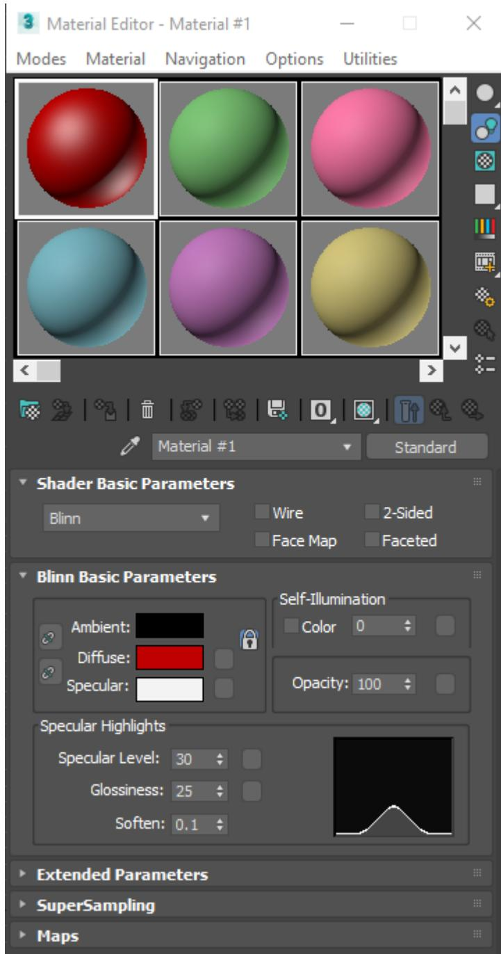
When creating lines for laser display, Lasershow Converter MAX gives you the option of using the material's **Ambient color**, **Diffuse color**, or **Specular color**. In addition, you can select a **Custom color** that you want the lines to be, regardless of the color of the object's material.
