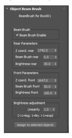
Beam Brush is dynamic beam divergence technology manufactured by the ScannerMAX division of Pangolin, and included in certain projectors manufactured by Kvant. The Beam Brush features of the Lasershow Converter MAX plug-in allow you to effectively map the Z-axis coordinate data from 3ds Max onto the beam diameter found in the 3ds Max objects. Each object can have its own Beam Brush settings, providing tremendous power and flexibility.
