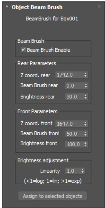
Beam Brush is dynamic beam divergence technology manufactured by the ScannerMAX division of Pangolin, and included in certain projectors manufactured by Kvant. The Beam Brush features of the Lasershow Converter MAX plug-in allow you to effectively map the Z-axis coordinate data from 3ds Max onto the beam diameter found in the 3ds Max objects. Each object can have its own Beam Brush settings, providing tremendous power and flexibility.
