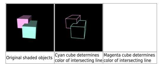
By default, Lasershow Converter MAX will favor the color of the object drawn first. However, you can control this on an object-by-object basis using the Color of intersecting lines drop-down list. The options available in this list are:
