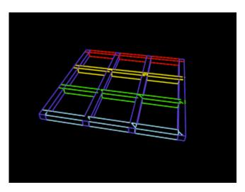
Because the beams are aligned so perfectly, it is impossible for Lasershow Converter MAX (or even the scanline renderer) to determine which surface is on top. The result is that stray lines appear in certain frames.
