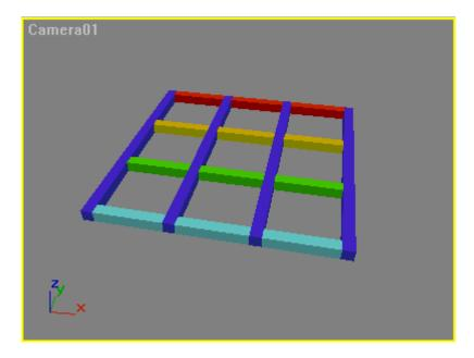
The height, width and length of the red, yellow, green and cyan beams were decreased ever so slightly. This allows the renderer to determine that the surfaces of the blue beams is on top of the surfaces of the other beams.
