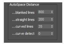
Note that in both cases, the **Straight lines** point density needs to be decreased from the default value of 300. This ensures there will be enough points placed for small details and to avoid rounding in the images.
