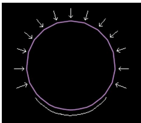
Although the corner detector will no longer put any extra corner points here, the curve detector will still place more points in this area. Moreover, as the camera angle changes, the facets will show up in different places and in different amounts of curvature.
