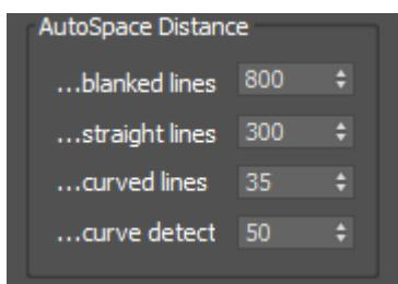
A better setting for this situation is shown below. It reduces the difference between the **Straight lines** and the **Curved lines** point density. This ensures there won't be as many radical changes in point density as the curvature changes. In addition, reducing **Curve detect** reduces the sensitivity to curvature changes.
