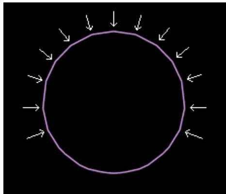
Depending on your point spacing settings, the angles between the facet lines might look like corners. If you allow corners of wide angles to be detected by Lasershow Converter MAX, you will no longer get a nice round laser path. Instead, you will have a polygon with sharp corners. There are two ways to make a coarsely meshed object always produce a round outline.
