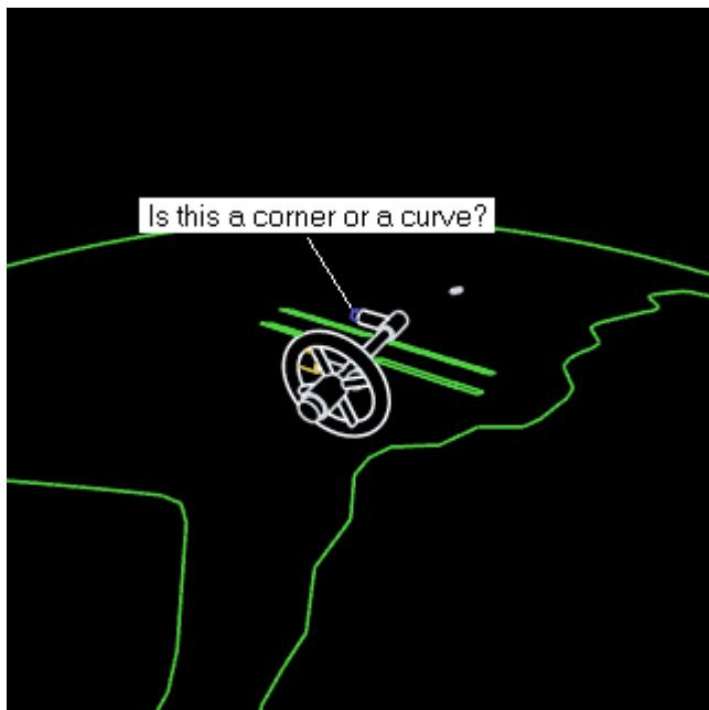
If you look closely at the picture below, you can see that the curved part of the mount is actually made up of line segments at angles to each other. If you have **Corner points 155-165°** set to a value of 1 or higher, Lasershow Converter MAX will detect this as a corner instead of a curve. Ordinarily you could fix this by simply setting **Corner points 155-165°** to 0.
