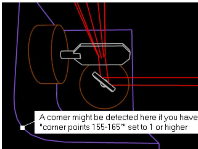
But what if there were instances where you wanted extra corner points at angles between 155 and 165 degrees? In this case, you can tell Lasershow Converter MAX that you still want corner points at these angles, but reduce the corner detection sensitivity by setting **Corner detect** to a lower value such as 10.
