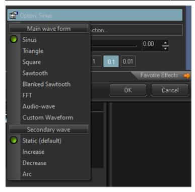
Under option dropdown, you can change the wave type, including: Sinus, Triangle, Square, Baked Sawtooth, FFT (for inputs), Audio-wave (for audio input) and custom waveform to draw your own waveform.
