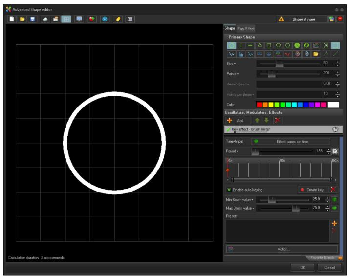
Brush limiter will change the minimum brush value of the frame, and maximum value of the frame. This can be used to change the brush value of an object without overriding previous brush effect values like color type brush effects. This modifies all points Inside the frame.
