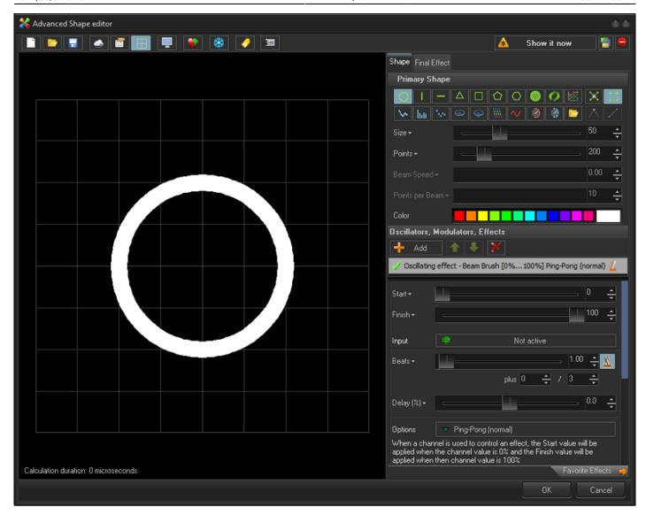
Beam Brush® (Oscillating effect type) will modify all points brush value. Using the start to finish values, you can animate between these values repeatedly over the time set in the beats, or seconds slider. You can also use the delay slider to change at what point the animation will start.
