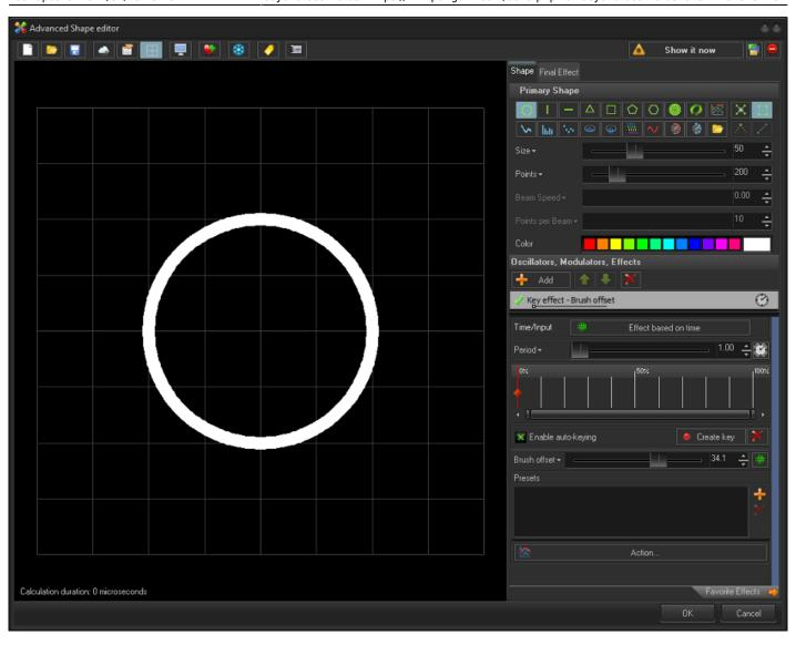
Brush offset will shift the total brush value of each point in the frame based on the value in the key.
