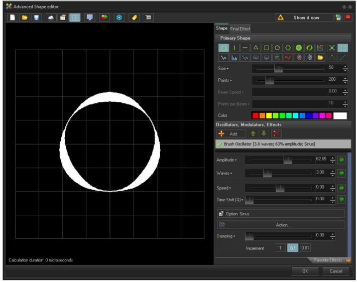
Beam Brush® Oscillator is an effect which will modify the Beam Brush® value of points in a shifted wave pattern. You can control the amplitude, which is the brush value maximum the wave will go. You can change the number of waves total over all points. You can change the speed of which the waves will move through the points. You can shift the start time and position of the waves.
