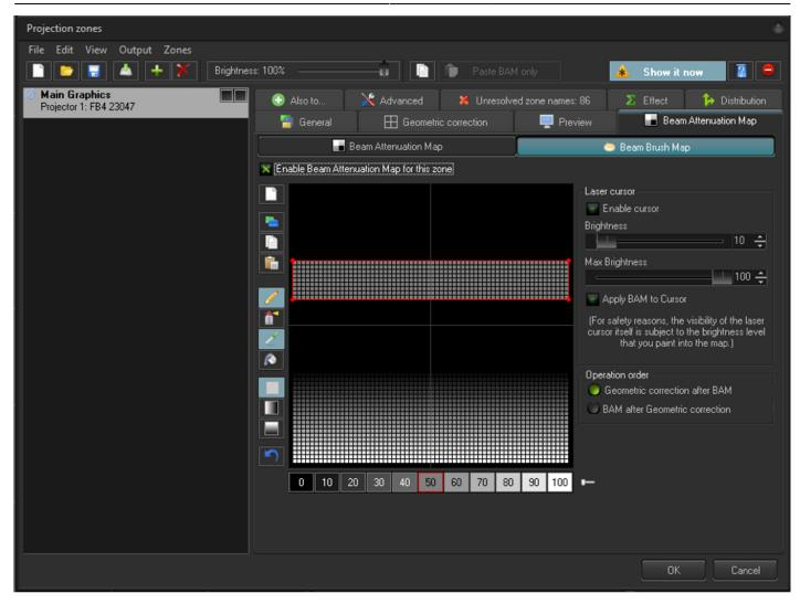
The Beam Brush® map is in projection zones, under "Beam Attenuation Map". We have added a second option which is called the "Beam Brush Map". This works incredibly like the regular Beam Attenuation Map, however instead of overall brightness, we are controlling the percentage of Beam Brush® used.
