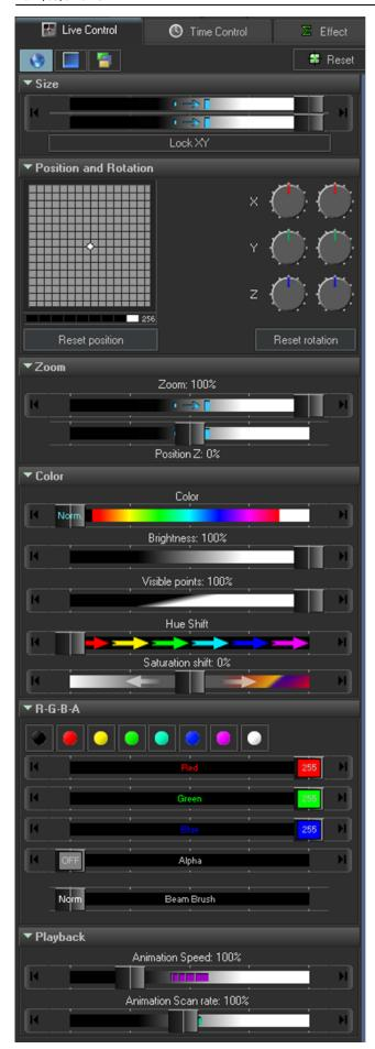
The Live control tab is where you can control overall parameters of your content as a global override and is the values you would change when you run a midi controller.
