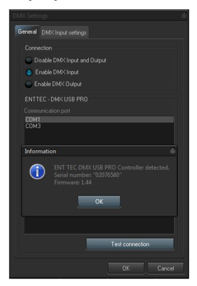
First specify whether you want to use DMX Input or Output using the "Connection" portion of the dialog box. After that, specify the COM port where the DMX-to-USB controller is connected.
