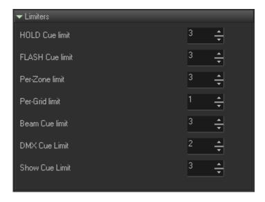
There are two set of Limiters, the first is for One Cue mode, the second for Multi Cue mode. The logic of Limiters is in some cases corrected by practical experience. The system should give the expected results in the most cases, although there can be tricky combinations, in which case Limiters are useful.
